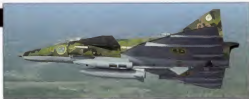
Displaying its 'chisel' nose, this Viggen is equipped with a Red Baron reconnaissance pod on its forward fuselage station.
